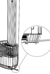
Do not use/start the device if the salt balls get into the fan housing!
