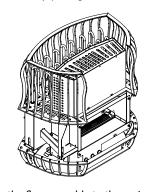
**5.** Fix the flue assembly to the main frame using 4 bolts included in the set.
