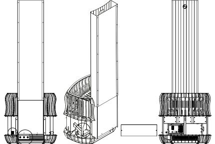
**NB!** Due to the potential danger of thermal embrittlement, it is forbidden to use a PVC-insulated cable as the connection cable for the sauna climate device.
